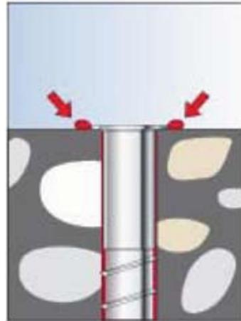
**4. Make sure screw is flush with the surface and epoxy exits the top of the drill hole.**
